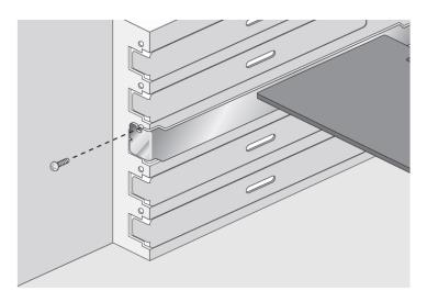
Figure 6. Securing the Adapter Card
